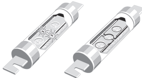
Fuse During Fault
